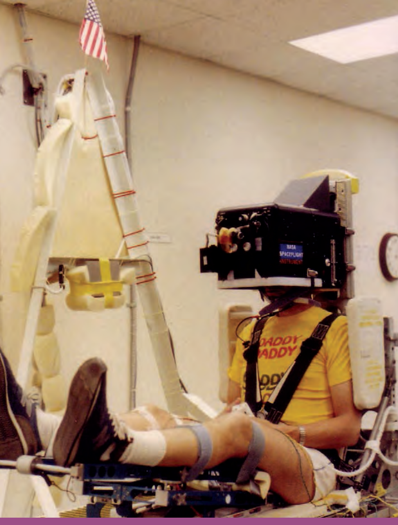
For Spacelab's 1983 maiden voyage the MVL prepared experiments to measure changes in astronaut balance. Crew member and MIT/MVL alumnus Byron Lichenberg (SM '75, ScD '79) is shown here during pre-flight acceleration on the lab's "vestibular sled." Instruments inside the box-like helmet measure his eye movements and movement perception. (MVL)
