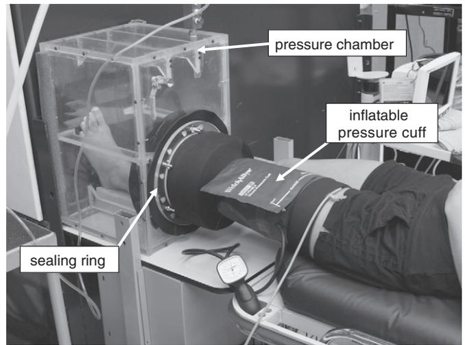
Fig. 2. Pressure chamber with neoprene pressure seal and sealing ring.
