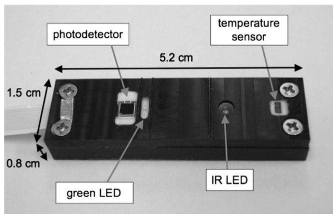
Fig. 1. Head stage of the PPG system showing the green and infrared (IR) LEDs, as well as the photodetector.
