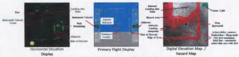
Figure 3. Three displays used for lunar landing
