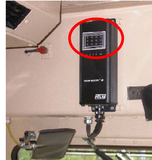
EMD F40 cab retrofit with Train Sentry III visual alert above forward view
