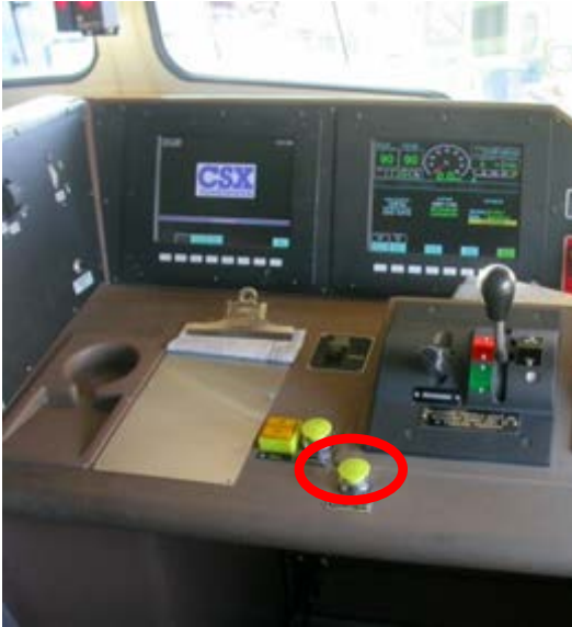
EMD SD70 cab console with software alerter. Timer reset button circled.
